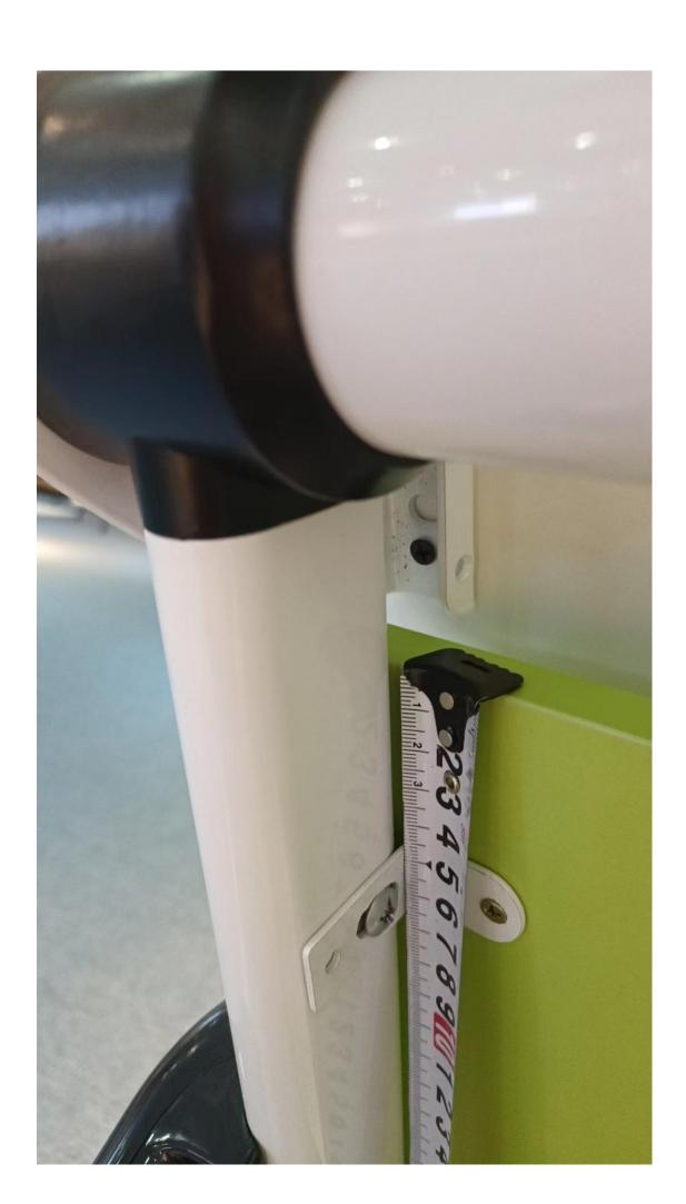
baffle exposed baffle "ears" 4.5 cm on the line
