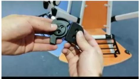
put the two accessories together and rotate the left movable buckle can be to lock
